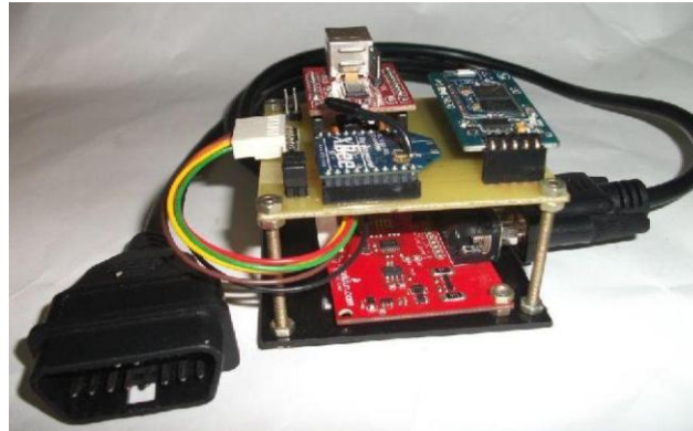
Fig.3 The Transmitting end hardware assembly: The OBD to UART board integrated with the zigbee module, Bluetooth module and USB to RS232 breakout module.
