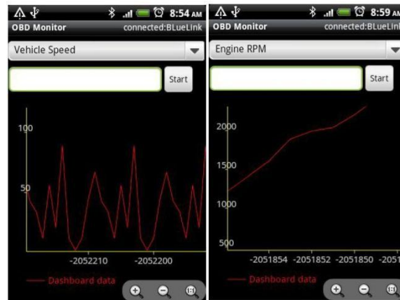
Fig.7. The Android app running on HTC Wildfire S phone (Android 2.3 Gingerbread) displaying real-time ECU data (Vehicle Speed, Engine RPM)
